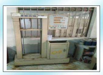
**Elastic Stretchability Test**Jacquard elastic elasticity test
